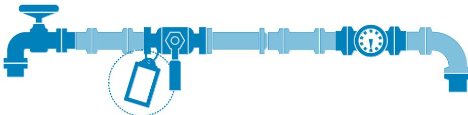
2. WATER SHUT-OFF VALVES SHOULD BE TAGGED/PLACARDED AS WORK PROGRESS
